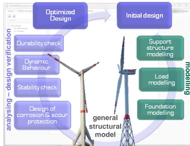
Fig. 4 Optimisation potential in design process
