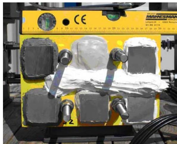
Fig. 2 Test coupon with online monitoring
