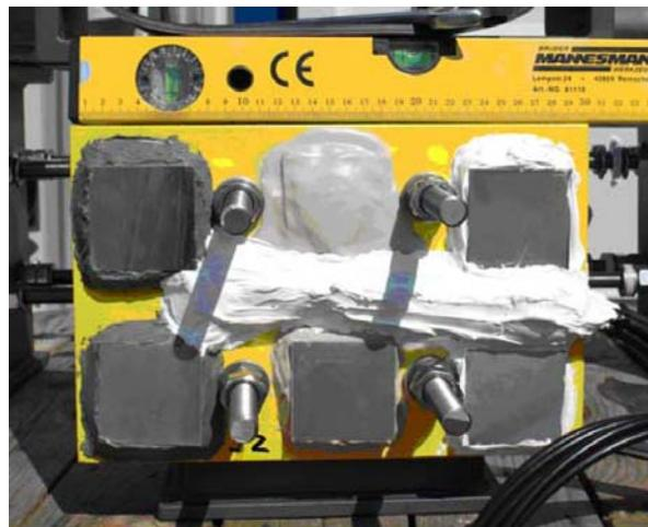
Fig. 2 Test coupon with online monitoring
